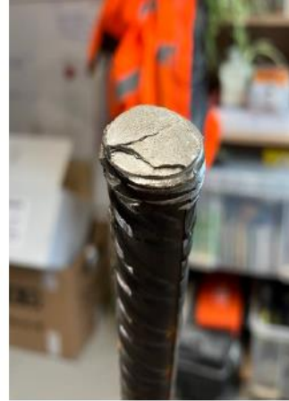
Photo 3: Sheared failure at threaded section
