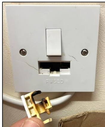
Center photo: Shows scorch marks may be from a loose contact at the fuse connection point. The longer the heater is on, the hotter the loose/poor connection gets.
